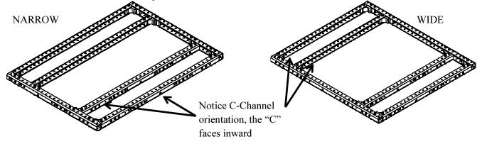
Step 5: Place the axles as shown in the picture below for the NARROW base and tighten them with the 3/8" nylon nuts.
